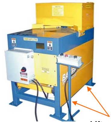
Lift points under the main frame from either side of machine
