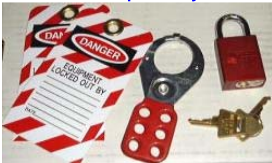
Example of lockout tags, lockout hasp and keyed lock
